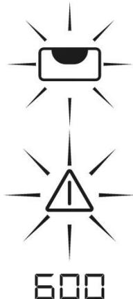
The levelling indicator flashes on the lit display. If the tripod head is sloping by more than 5°, this is indicated by the laser beam flashing quickly and the alarm symbol being displayed. In this case, switch off the unit and align the tripod more carefully. Once horizontal levelling is completed, the laser beam starts to rotate.
