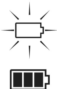
If the three bars on the display are blank and the outside frame flashes, the battery is flat and you must charge it. If you do not notice this, the device switches off automatically after a certain amount of time.
