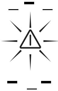
If the traverse path is exceeded while aligning, this is indicated by a change in the arrangement of the bars, by a quickly flashing warning symbol and by the laser beam.
