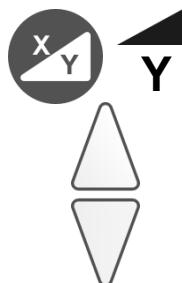
2nd key press: X - Symbol disappears but slope symbol and Y is shown in the display.
