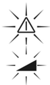
If external influences (shock or temperature) change the position of the device, the system interrupts rotation and the laser beam, the slope and the warning display flash rapidly.
