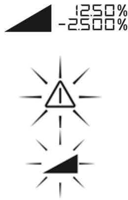
If external influences change the position of the device, the Autoslope monitoring system registers this and automatically initiates adjustment. If the device is tilted a relatively long way, the system interrupts rotation and the laser beam and the warning display flash rapidly.
