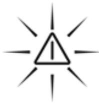
In the case of major changes to the mounting position (e.g. accidentally moving the tripod leg), a TILT function ensures that the device switches off and draws attention to the fact by the laser beam and the warning triangle flashing quickly.
