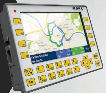
The rapid **MOBA Operand** with quad-core processor displays both order and measurement data directly in the driver's cab and makes them available for immediate processing. Thanks to the open operating system WindowsCE, the on-board computer is compatible with all common management software and can be incorporated into any installation quickly and easily.
