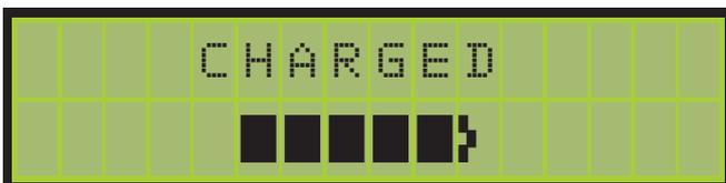
When the battery has been charged for 6 hours it will display CHARGED.
