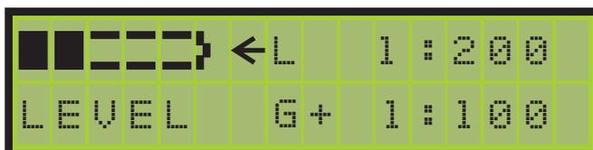
Indicates in ratio format, the distance line is to left (L) or right (R) of centre.
