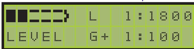
Indicates in ratio format the distance the line is to left (L) or right (R) of centre.
