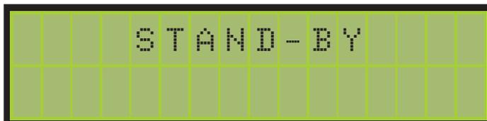
When the laser is in standby mode, this message will appear and the LCD back-light will blink approximately every 2 seconds.
