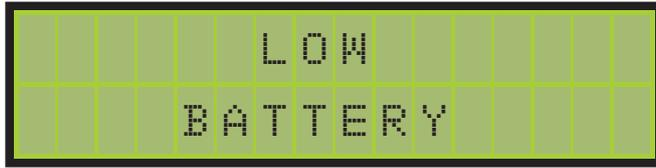
Should this message appear when the laser is switched on, the internal battery voltage is too low for accurate operation.
