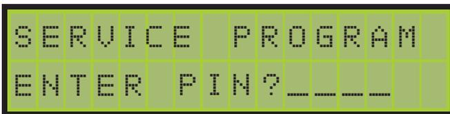
A four digit PIN number must be entered to continue. Correct PIN 1234 must be entered within 5 seconds or LCD will return to normal mode.
