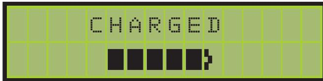
When the battery has been charged for 5 hrs or the internal voltage is greater than 10.0 V, the fast charging ceases and trickle charging commences.
