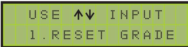
Operate the “GRADE INPUT” key to reset grade counter to 0.000%. The LCD will display “EXECUTED” when this occurs.
