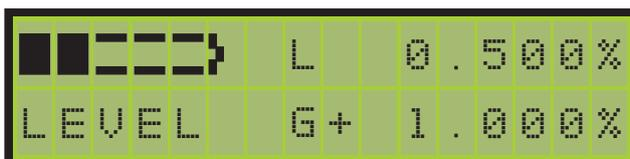
Indicates % of grade (G) and if positive (uphill) or negative (downhill). The word 'LEVEL' indicates that laser has selflevelled.
