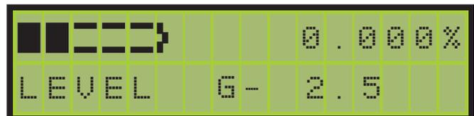
4. Press the Grade Input key again and the laser will begin to adjust to the desired grade.
