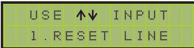
Operate “GRADE INPUT” key to reset the line counter to 0.000%. The LCD will display “EXECUTED” when this occurs.
