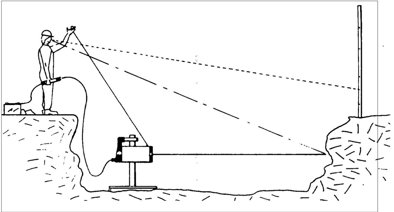
1. Dial the required percentage grade (%) into the Pipeguide.
