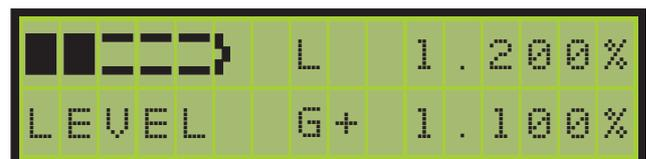
Indicates grade (G) in ratio format. The word 'LEVEL' indicates that the laser has self levelled.
