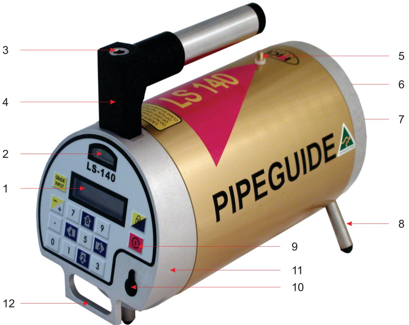
1. Liquid Crystal Display (LCD) with back-light (automatic)
