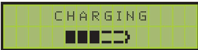
If the PIPEGUIDE is connected to an external power source and the on/off switch is off, the internal batteries will start to charge and this message will appear. If the PIPEGUIDE is connected to an external power source and is powered off the internal batteries will start to charge and this message will appear.
