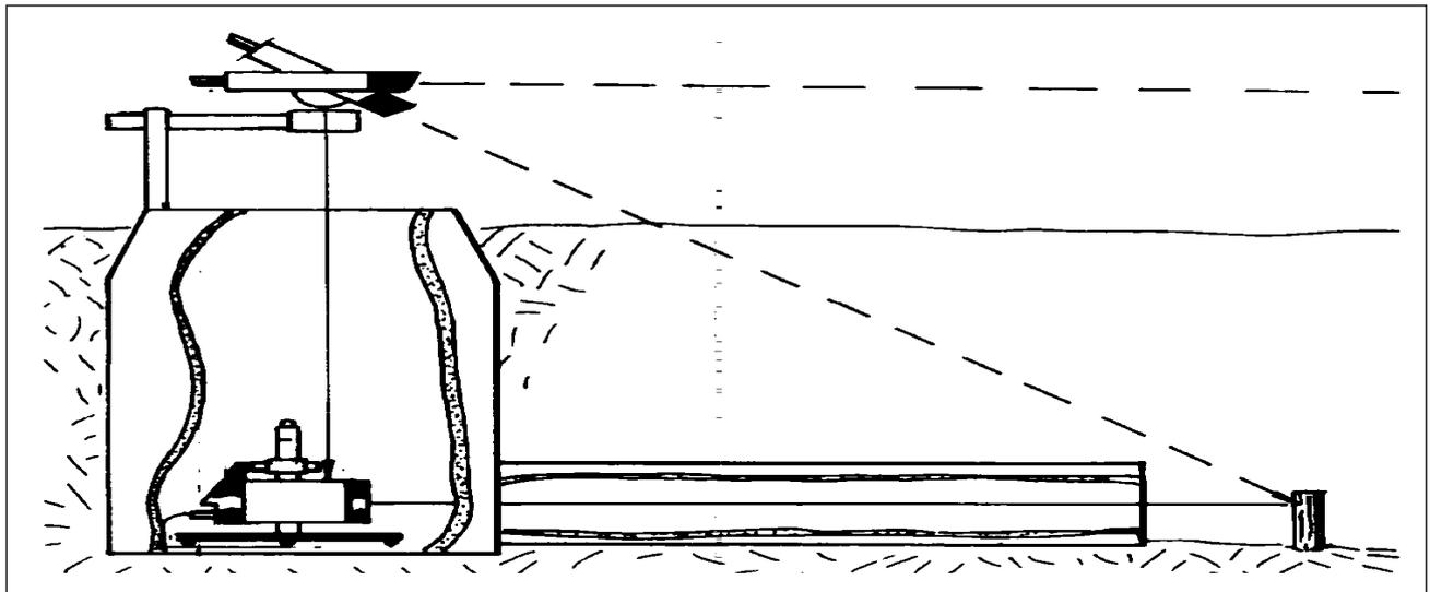
1. Plumb optical instrument over a known point or line of trench.
