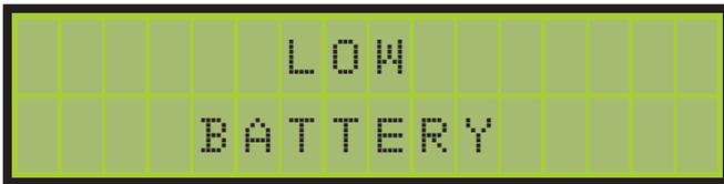
LOW BATTERY. This appears when the battery voltage drops below safe operating level while the laser is being used.
