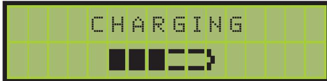
If the Pipeguide is connected to an external power source and is powered off,, the internal batteries will start to charge and this message will appear. The LCD back-light will remain on during the charging process.
