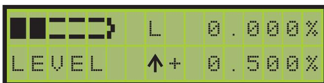
Indicates direction the beam is moving and the % grade of current position.
