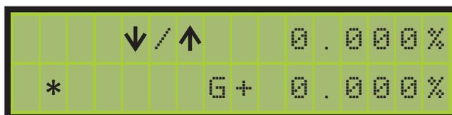
Indicates Pipeguide is tilted to the right.
