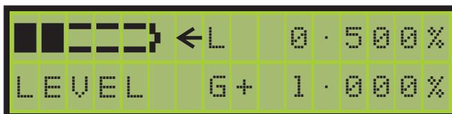
Indicates the direction laser is traversing and whether left (L) or right (R) of centre.
