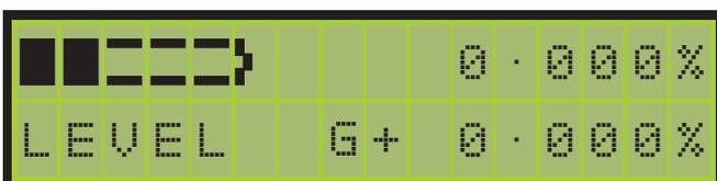
Internal battery voltage indicator. Indicates the charging status of the internal rechargeable battery.
