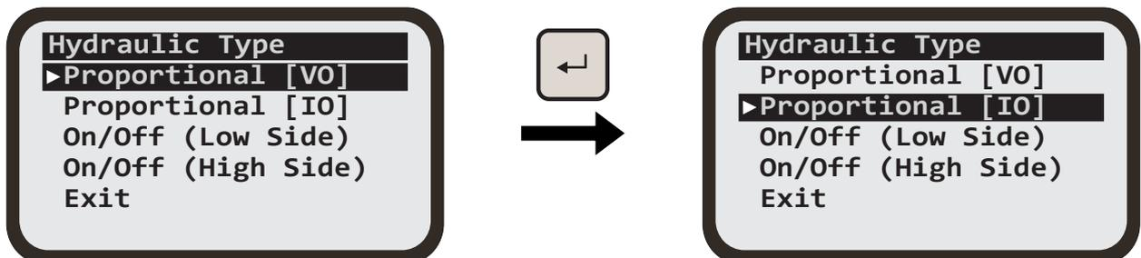
When finished, use [AUX] key to select 'Exit' and press [ENTER] key.
