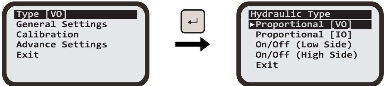
Using [AUX] key, select the type of hydraulic connected on the machine then press the [ENTER] key to set.
