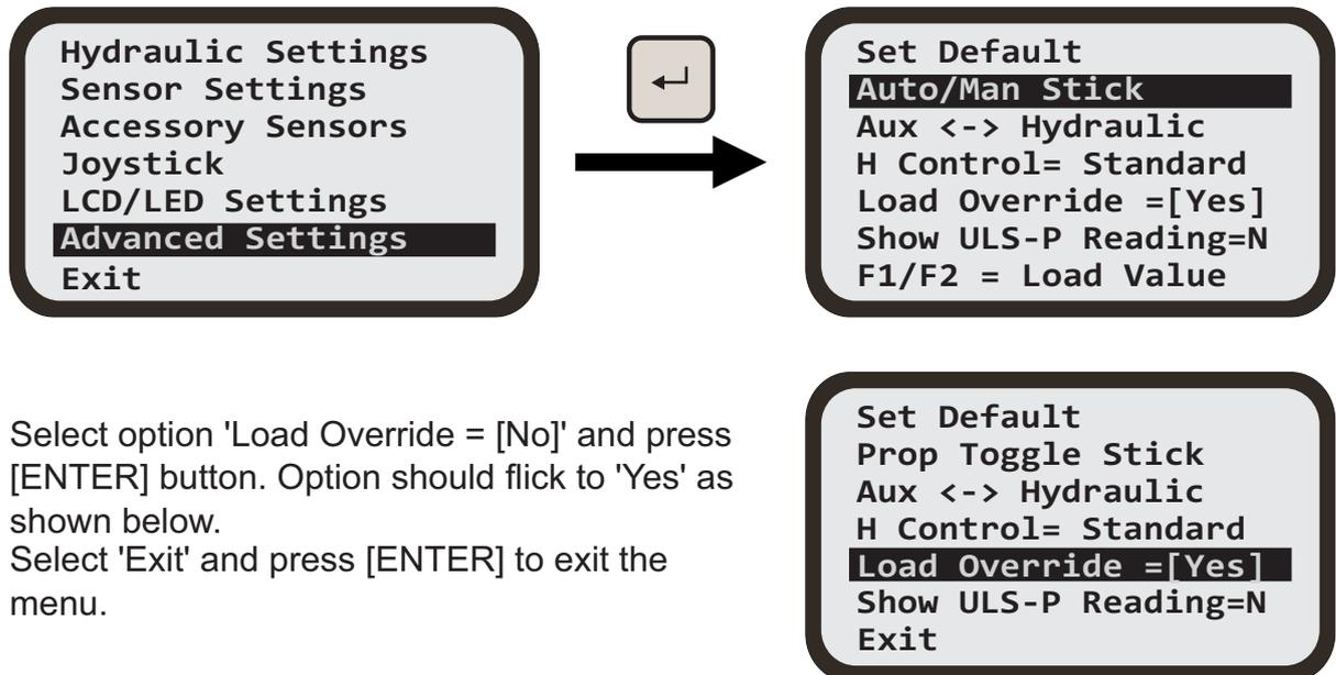
Select option 'Load Override = [No]' and press [ENTER] button. Option should flick to 'Yes' as shown below.
