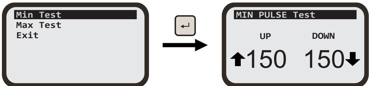
When doing Min Pulse Test, the aim is to find the minimum setting which will move the blade or bucket by the smallest amount in both upward and downward direction.
