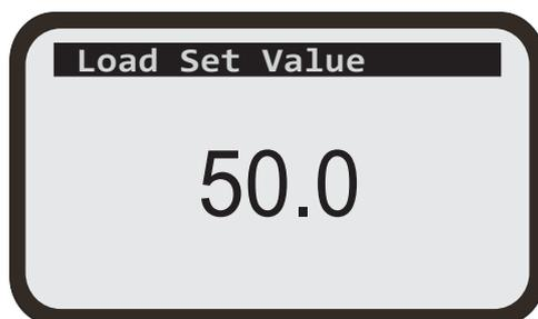
Use the [FUNC] up or down buttons to adjust the threshold to the desired level. The display returns to the standard screen after a few seconds of user inactivity. The desired level is usually job dependent and is determined by the user by trial and error at the start of a new job.
