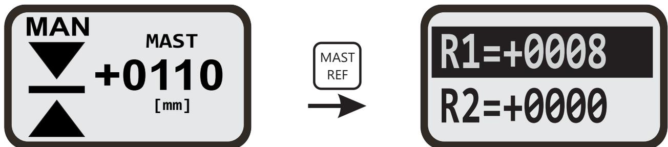
After selecting a reference slot press [ENTER] key and the selection will flash. Use [AUX] key to select and set a new reference point, then press [ENTER] key to confirm the new reference point setting.
