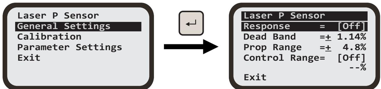
Select 'Dead Band' then press [ENTER] key. The selection will flash. Use the [AUX] Up/Down button to set the desired value.
