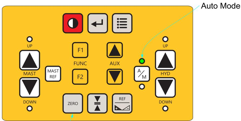
Press to zero the mast reference and current offset.
