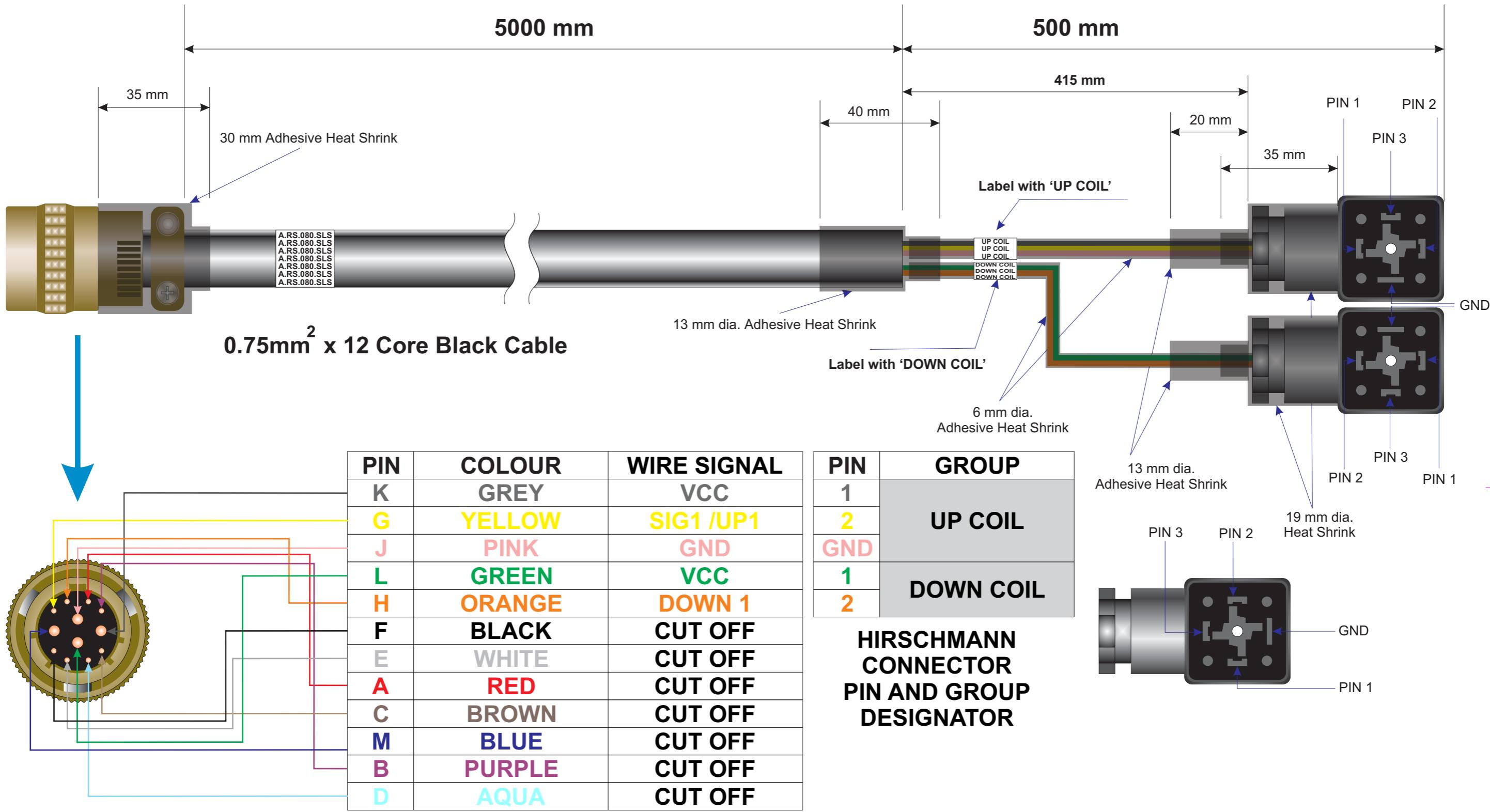
**Note1:** Adhesive heat shrink over connector shell and groups of wires.
